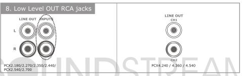
The LINE OUT allows you to build multiple amplifier systems without having to use splitter cords to distribute the signal. Now it is simply a matter of bringing one set of RCAS into the first amplifier, then using the line out RCA jacks as the feed to the next amplifier.
