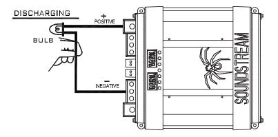
To Discharge the capacitor: With battery power disconnected, place the light bulb or resistor across the capacitor's positive and negative terminals until light goes out or for three minutes if using a resistor.
