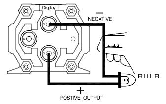
To Discharge the capacitor: With battery power disconnected, place the light bulb or resistor across the capacitor's positive and negative terminals until light goes out or for three minutes if using a resistor.
