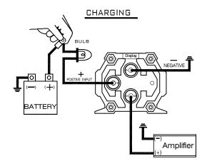
3. Place the supplied charging bulb between positive terminal of the capacitor and the battery's positive terminal. Do this for 2 ~ 3 minutes until the charging bulb goes out.
