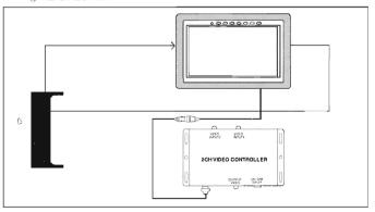
(§) Put the separator(§) between Monitor and Headrest when you separate the Monitor from headrest kit
