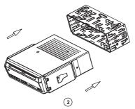
3. Mount the frame (accessory 11) and check that it is hooked to the unit.
