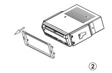
3. Remove mounting bracket 2 with screwdriver.
