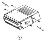
2. Hitch the mounting box(accessory 1) to the unit from rear to front.
