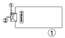
2. Replace the button cell with new one and make sure polarity is correct.
