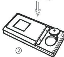
3. Push the holder back. Using the finger to push in the holder back until the locking sound is heard.
