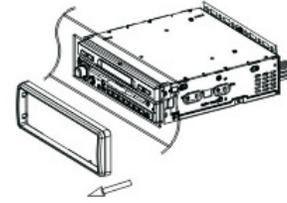
2 Unscrew the unit off the car on the two sides.
