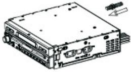
2 Tighten the back strap onto your car inside the dashboard.
