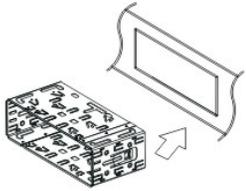
2 Bend the claws into place to secure the sleeve.
