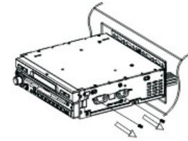
3 Unscrew the Nut M5 screw on the rear side of the unit and pull out the unit.
