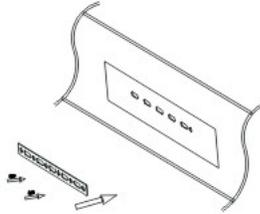
3 Place the unit into the dashboard; make the bolt bar across back strap; and then fix the bolt by the Nut M5.
