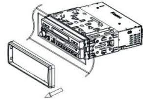
2 Insert the keys into the aperture between the unit and the mounting.
