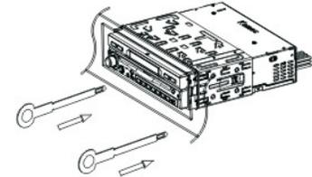
3 Pull the unit out of the mounting sleeve.
