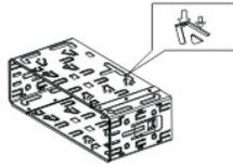
3 Slide the units into the mounting sleeve.
