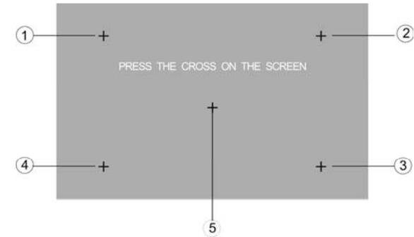
To touch the points from 1 to 5 until the points change to next cross by using a ballpoint pen or pencil. After all 5 points have been touched, the unit has been finished the CALIBRATION. If the calibration is succeeded, the unit would display the following page and then power off automatically.
