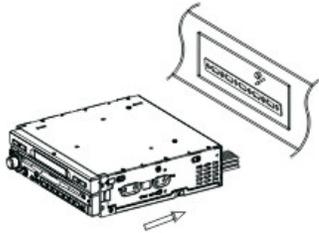
4 Screw the unit on the car on the two sides with M5x5 SCREWS.
