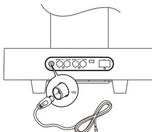
If reception is poor, connect the outside antenna.
