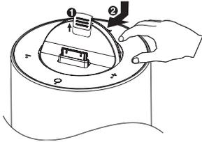
2. Raise up the buckle ❶, and rotate the dock module to original position ❷.
