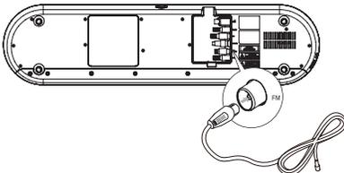
If reception is poor, connect the outside antenna.
