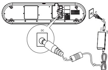
Connect the power adaptor to the DC socket on the unit and a wall outlet.
