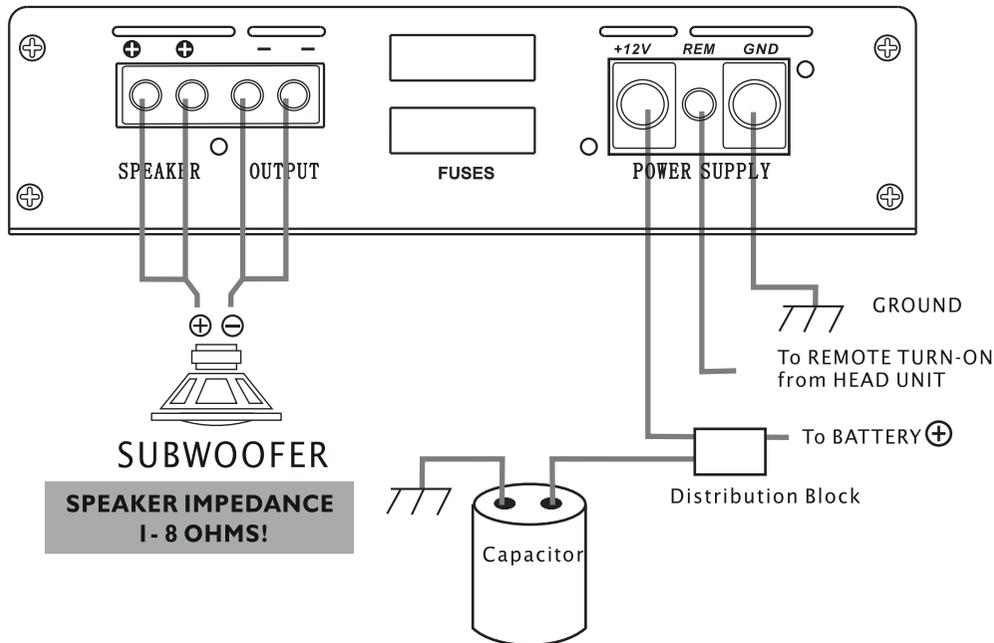
**NOTE:** The amplifier may receive its input signal from a head unit or signal processors subwoofer output.
