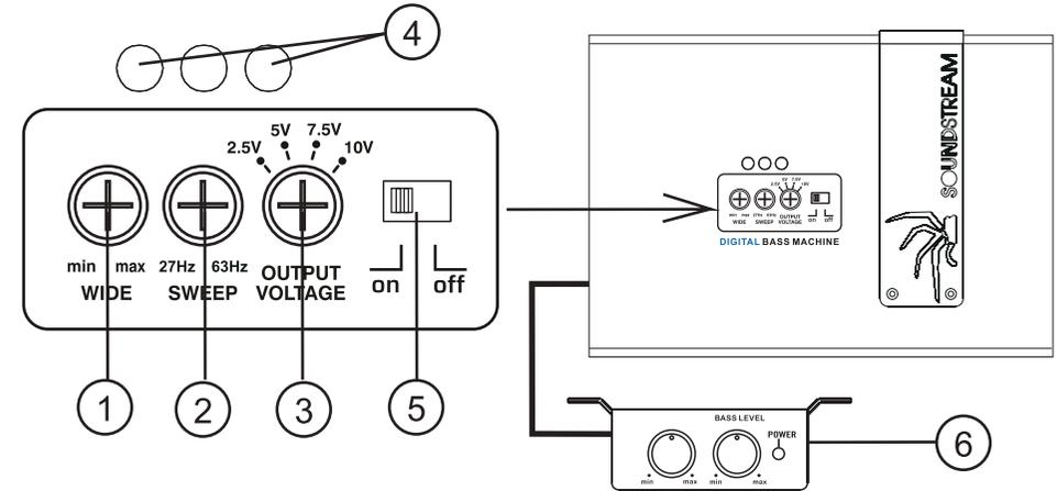
**1. WIDTH** increases or decreases the band width range, or "Q" boosting frequencies near the "center frequency." Narrow Q focuses on harmonics immediately surrounding the center frequency. Wide Q unlock harmonics all around the center frequency.
