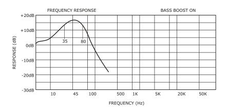
NOTE: Raising the Bass frequency allows higher frequencies to reach the bass speakers while blocking lower frequencies from midrange speakers. Lowering the Bass frequencies allows lower frequencies to reach the midrange speakers while blocking higher frequencies from bass speakers.
