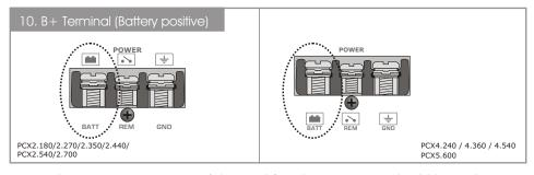
Due to the power requirements of the Amplifier, this connection should be made directly to the positive(+) terminal of battery. For safety measure, install an in-line fuse Holder (not included) as close to the battery positive(+) terminal as possible with an ampere rating; not to exceed total value of fuses in Amp.
