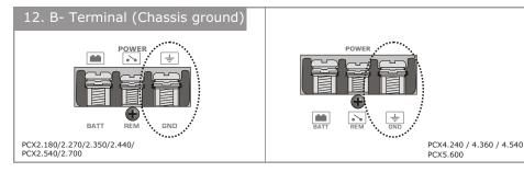
To avoid unwanted ignition noise caused by ground loops, it is essential that the Amplifier be grounded to a clean, bare, metal surface of the vehicles chassis.
