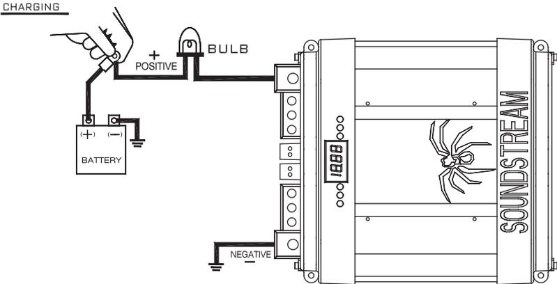
To Discharge the capacitor: With battery power disconnected, place the light bulb or resistor across the capacitor's positive and negative terminals until light goes out or for three minutes if using a resistor.
