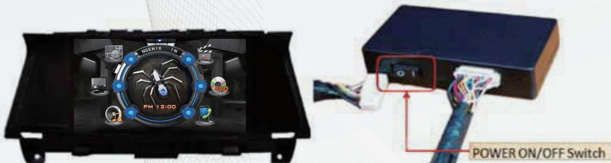
→ Honda Model has Power On/Off switch back side of Control box.
