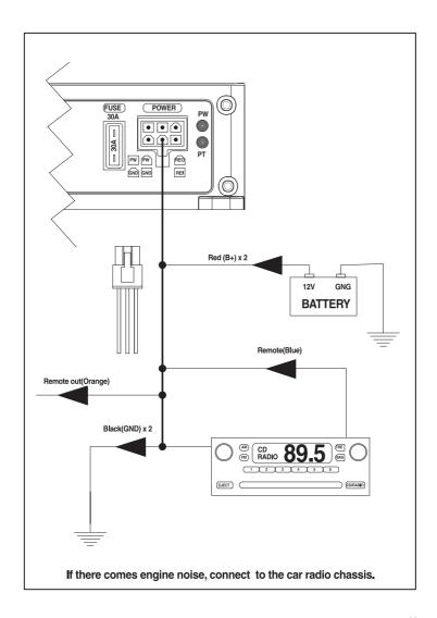
These amplifiers are designed to work within a 10 to 16.8 volt DC range. Before any wires are connected, the vehicles electrical system should be checked for correct voltage supply with the help of a voltmeter.
