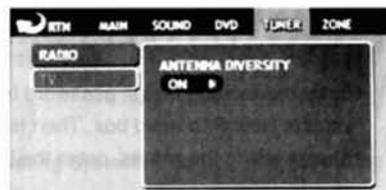
When set to OFF, only the antenna connected to antenna connector No. 1 is used.
