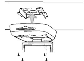
5. Flip the monitor screen down and tighten the monitor to the support bracket, using the supplied screws.
