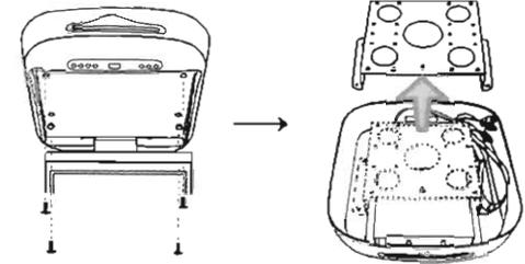
3. Tighten the metal support bracket to the ceiling support beam(s), using the supplied screws. Take extra care to not penetrate the roof of your car. The arrowhead symbol on the support bracket should point toward the rear seat(s) when installed.
