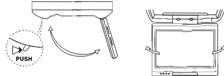
※ The monitor will automatically turn off when it is closed to the ceiling mount. When the monitor is opened again, it will automatically be turned on.
