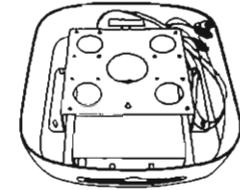
2. Disassemble the metal support bracket from the unit as shown in the illustration, by unscrewing the four screws on the unit body.
