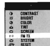
3. Press the arrow (UP/DOWN) buttons to select a setting between 88.3, 88.5, 88.7, 88.9, and 90.1MHz.
