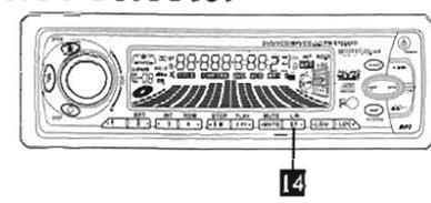
4. Press **14** (ST, L/R) button to select MONO mode or STEREO mode.
