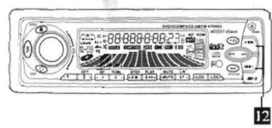
1. **Manual Tuning:** Press **12** (+) or (-) button continuously to select a station upward or downward respectively.
