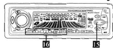
5. Press **15** (AMS) button to scan each stored station 10 seconds respectively which stored in **16** (1~6) number buttons. When AMS mode is carried out. "INT" appears on display. (See the picture). You also can press the corresponding number button or AMS button when your desired station is charged. It starts playing that station.
