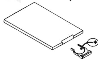
3. Insert the Battery Holder into the Remote Control.
