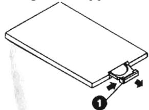
2. Put the button-type battery(+) mark upward into the Battery Holder.
